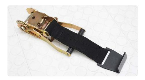
STEP 17 | If the hook is face the wrong direction or needs to be changed, remove the bolt on the tie down using a 15 and 17mm wrench, flip the strap around, and reinsert and secure the bolt.
