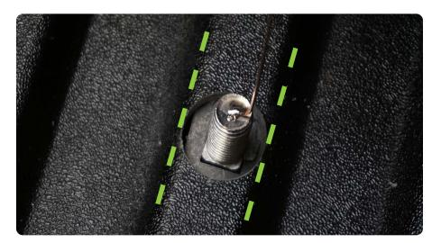
STEP 9 | Insert the plastic retaining plate and drop it down the wire. Spin plastic until bolt is secured to the bed.
