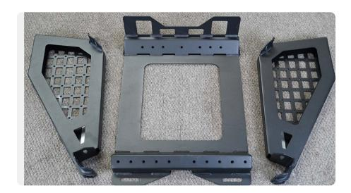
STEP 2 | Use the provided M8 hardware and a 5mm Allen to loosely secure side onto the base plate.
