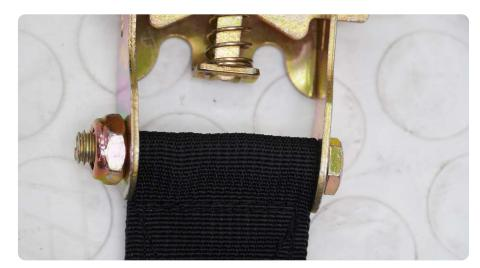
STEP 18 | Tighten the strap until tight and tire is secure and double check strap tightness after 24 hours of driving.
