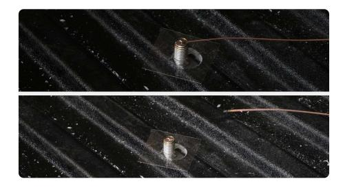
STEP 11 | Place the carrier over the bolts. Secure the carrier in place using the provided M12 washer and nylon locking nut using a 19mm socket.
