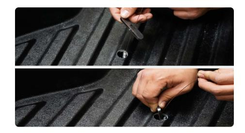
STEP 8 | Once the plate is in the hole align the plate and the carriage bolt.
