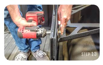
STEP 14: Next using the same 19mm socket and wrench, tighten the bottom of the vertical carrier to the bottom main rail.
