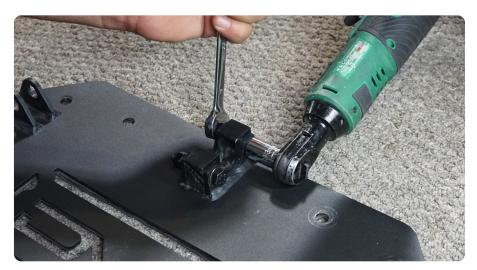
$\begin{array}{c|c} \text{STEP 13} & \text{Install the backing plate} \\ \text{to the tailgate of the vehicle using the} \\ \text{factory hardware and a 13mm socket.} \end{array}$
