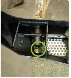
$\begin{array}{c|c} \text{STEP 15} & \text{I} & \text{Install the provided spacer} \\ \text{plate, followed by the bearing as shown.} \end{array}$
