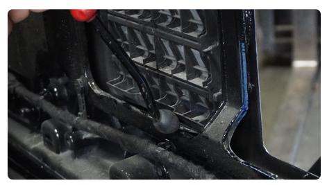
STEP 8 | Using a Dremel or cutting tool of choice, remove the three sided border from the fin vents.
