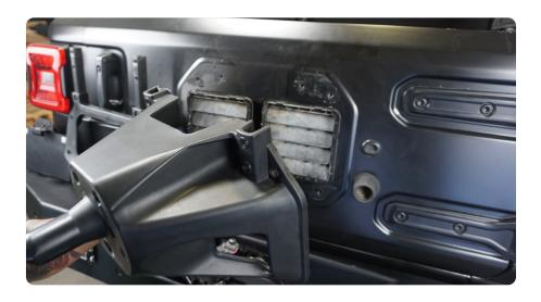
STEP 6 | Open the tailgate and use a trim clip tool to remove the plastic panel from the tail gate.
