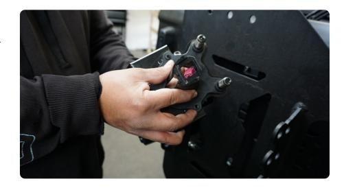
STEP 25 | Reconnect the rear camera harness to the rear camera.
