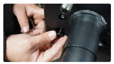
STEP 32 | Adjust the camera tube and secure using the provided M6 hardware with a #4 Allen bit.
