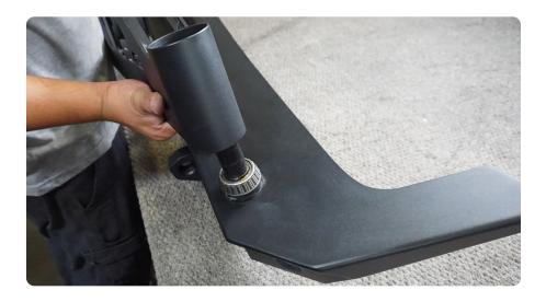
STEP 19 | Install the upper race and remaining bearing as shown with the race being placed first, and the bearing on top, facing down.
