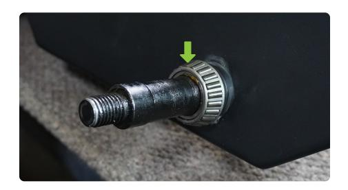
STEP 16 | Place the tire carrier on to a work bench upside down. Place the lower bearings race into the tire carrier as shown.
