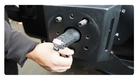
STEP 28 | Secure the factory rear camera/ tire mount to the DV8 Tire Carrier using the (2) factory torx head screws previously removed.
