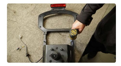
STEP 36 | Mount the DV8 tire mount onto the DV8 hinge/tailgate bracket. Using the provided M12 hardware, an 18mm socket and a 19mm socket, secure the tire mount in place.
