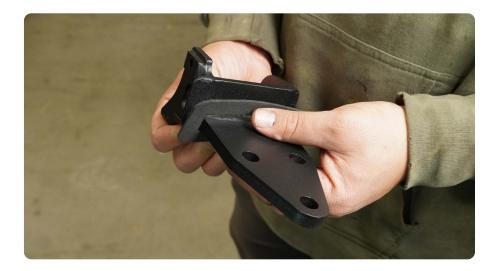
STEP 24 | Before mounting the DV8 hinges, place a small mount of blue thread locker to each of the (6) factory hinge bolts.
