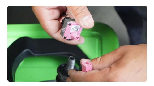
STEP 12 | If you vehicle is equipped with the newer camera style shown, depress the camera from the camera mount, unplug the camera harness and set everything off to the side.
