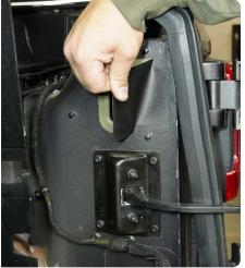
STEP 22 | Use a 13mm socket to remove the (6) factory hinge bolts. Set the factory hinges off to the side, they will not be reused.
