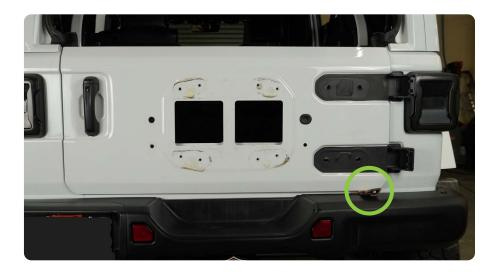
STEP 27 | While holding the metal sleeves in the tire carriers bushings mount the tire carrier to the hinges.
