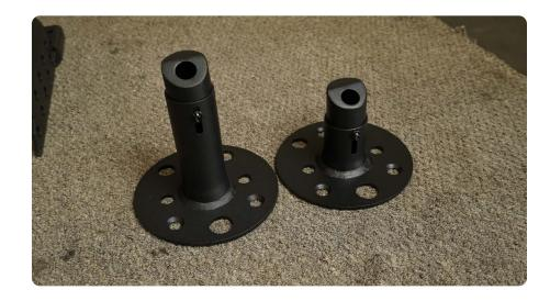
STEP 33 | Install the factory rear camera/camera housing and wheel stud plate on to the DV8 tire mount as shown.
