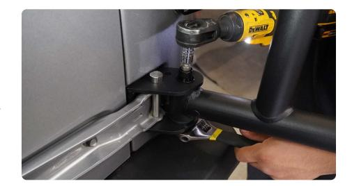
STEP 35 | Install the (2) M10 x35mm into the hinge brackets as shown. Do not tighten these down until after the carrier is adjusted fully in Step 46.
