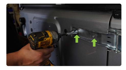
STEP 8 | Use a T50 Torx tool to remove the hinge to body mounting bolts.
