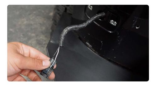
STEP 49 | Continue routing the extended license plate harness behind the tailgate cover into the tailgate and through the vent as shown.
