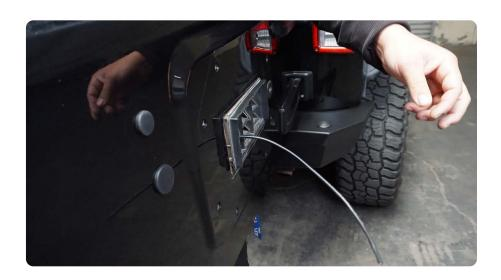
STEP 51 | Continue routing the extended over and into the tire carrier cage.
