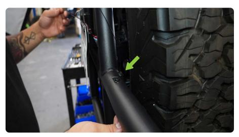
STEP 53 | The tire carrier cage is equipped with (2) 1/2 inch holes to mount additional accessories such as antennas, LED whips, flags and etc.
