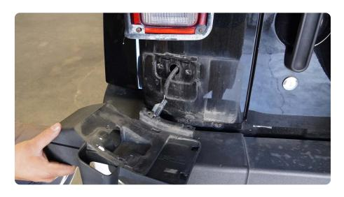
STEP 27 | Push the factory license plate light wiring harness back into the body of the jeep.
