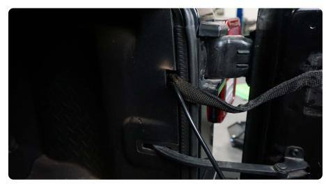
STEP 50 | Use zip ties to secure th third brake light factory wiring harness, it will not be used with the DV8 tire carrier.
