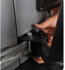
STEP 36 | Install the rubber cone on to the tire carrier spindle and the install the tire as shown.
