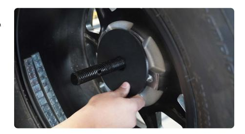
STEP 38 | Use the T handle to secure the spare tire on to the tire carrier.
