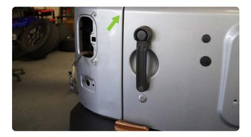
$\begin{array}{c|c} \text{STEP 18} & \text{Use a trim tool to lift the} \\ \text{hinge side of the tailgate up and align the} \\ \text{body lines.} \end{array}$
