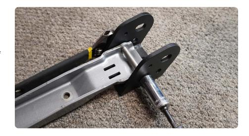
STEP 15 | Loosely mount the completed hinge assembly on to the vehicle using the provided M8x30 Counter sunk head bolts and a #5 Allen tool.
