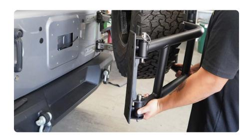
STEP 41 | While the tire carrier is still attached to the mounting bracket (not shown in photo) close the tire carrier and lay the bracket against the body of the vehicle and mark the holes that will need to be drilled out.
