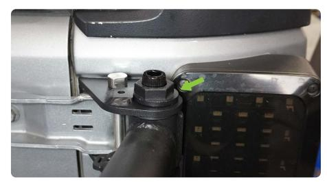
STEP 45 | Once the tire carrier is adjusted to the desired height, lock the cam bolt in place using a 12mm Allen tool and an adjustable wrench.
