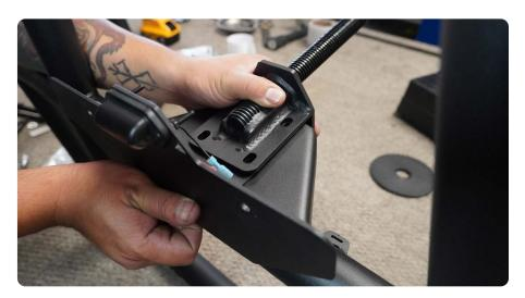
STEP 31 | Secure the license plate bracket and tire spindle to the tire carrier cage using the provided M8 hardware and a 13mm socket.
