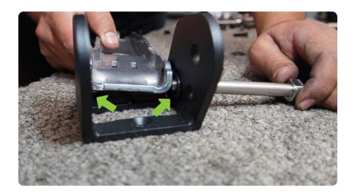
STEP 13 | Place a 1mm spacer on each side of the factory hinge to start and insert the provided hinge pin to check side to side spacing.
