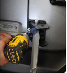
STEP 16 | Use a 13mm socket and the factory hardware to loosely secure the hinges to the tailgate.
