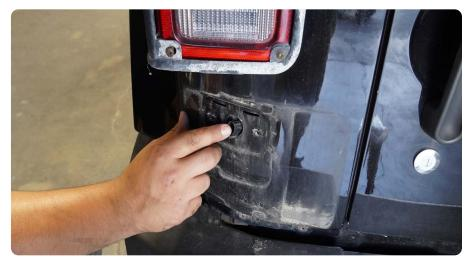
STEP 28 | Clean off any dirt from where the license plate housing was mounted and install the provided license plate cover.
