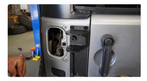
STEP 44 | Close the tire carrier. If adjustment is needed, turn the cam nut on the top hinge bolt to tilt the tire carrier up or down.
