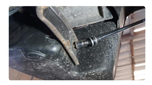
STEP 25 | With the bumper support disconnected you can flex the bumper down enough to use a 7mm socket to remove the housings (2) lower mounting hex bolts.
