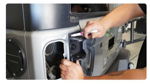
STEP 42 | Use a 3/8" drill bit to drill the marked holes into the body of the vehicle for the tire carrier bracket.
