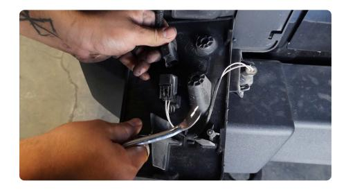
STEP 24 | To gain access to the housings (2) lower mounting hex bolts, use a 15mm socket to disconnect the bumper from the bumper support on the drive side only.
