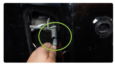
STEP 4 | With the light unplugged, push the rubber grommet holding the wire towards the outside (back) of the vehicle. Pull disconnected plug though hole in rear door.
