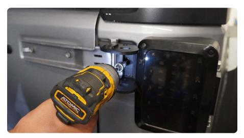
STEP 20 | Remove the driver side tail light at this time using a Phillips head screwdriver.
