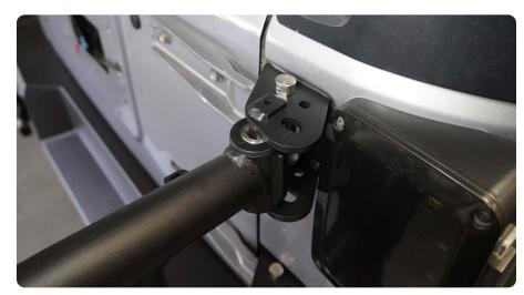
STEP 33 Using a 12mm Allen tool and adjustable wrench, loosely secure the tire carrier to the top hinge using the provided M14x34mm bolt, Cam nut, M14 flat washer and M14 nylon lock nut.
