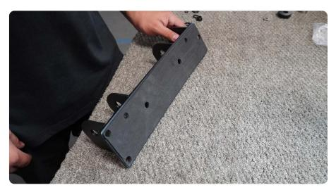
STEP 40 | Attach the driver-side bracket to the tire carrier using the provided pins.
