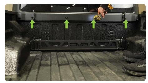
STEP 5 | Slide the tube tire carrier on to the drivers side, side mount with handle.
