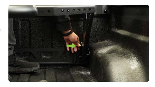
STEP 9 Using a 19mm socket. Lifting up slightly on the carrier, tighten the top (4) M12 bolts.
