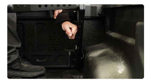
STEP 11 | Installing the shocks is easier with two people. Holding the carrier slightly above 90deg (flat with the bed floor), install the gas shocks that were provided.
