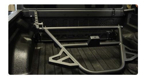
STEP 7 | Slide the passenger side bracket into carrier and install mount to the rear cross bar using M12x55mm bolts.
