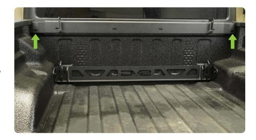
STEP 4 Use the provided (4) M6x30mm hex bolts and a 10mm socket to secure the center of the upper bracket to the bed panel.
