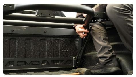
STEP 12 | Using a 12mm & 13mm wrench wrenches, tighten upper and lower mounts on both shocks.
