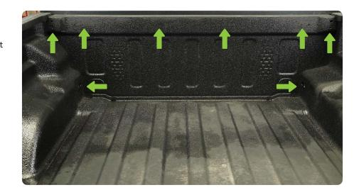
STEP 2 | Place the tire carrier base bracket in the truck bed as shown.
