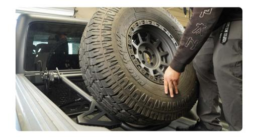
$\begin{array}{c|c} \text{STEP 15} & \text{Center the tire over the} \\ \text{post and insert the rubber cone into the} \\ \text{tire.} \end{array}$
