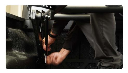
STEP 13 | Install the post onto the tire carrier mount using the (5) M8x25mm bolts using a 13mm socket.
