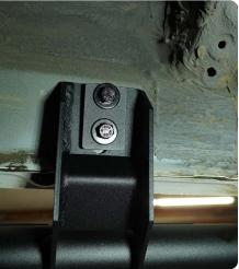
STEP 4 | Adjust the steps height level with the vehicle.
