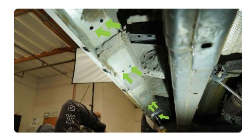
STEP 2 | With assistance, lift the step up to the vehicles rocker panel aligning the step with the factory threaded holes in the rocker panel.
