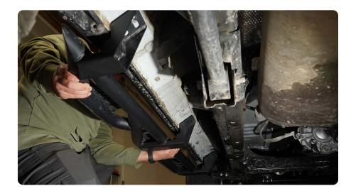
STEP 3 | With the step loosely mounted, center the step, side to side with the vehicle.
