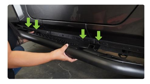
STEP 3 | Loosely secure the steps with the provided M8 hardware.
