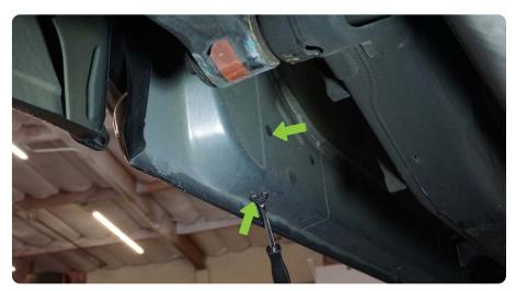
STEP 2 | With assistance, lift the DV8 OE Plus Steps up to the vehicle and use the provided M8x30 hex head bolts to loosely secure the steps in place.
