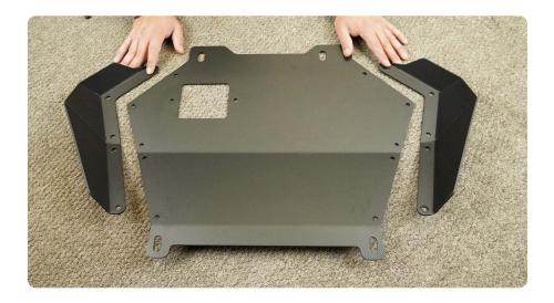
STEP 3 | Place the skid plate wings behind/on top of the skid plates center plate, use the (10) provided M8x20mm Allen head bolts to loosely secure the wings to the center plate.
