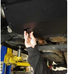
STEP 8 | Use the (2) provided M8x20 counter sunk Allen head bolts to secure the oil drain cut out plate in place.
