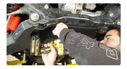
STEP 7 | Place the oil drain cut out plate into the skid plate at an angle, lay the cut out plate flat aligning the mounting bolt holes.
