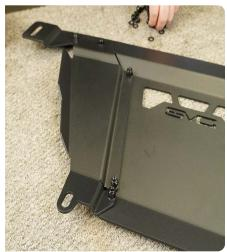
STEP 5 Use a #5 Allen tool and 13mm wrench/socket to secure the (10) M8x20mm wing bolts.
