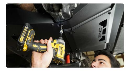
STEP 12 | Use an 18mm socket to secure SPTT1-08s front (4) mounting bolts.
