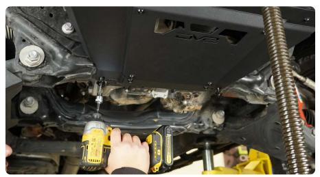
STEP 8 Use a #5 Allen tool to secure the (2) rear M8 mounting bolts.
