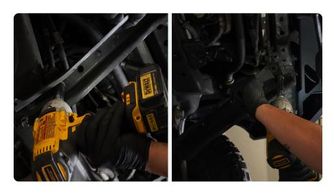
STEP 3 | With assistance loosely secure the skid plate using the factory hardware from the skid plate braces and a 17mm socket.
