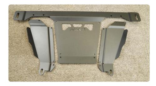
STEP 4 | Place the skid plates wings behind/on top of the center plate.
