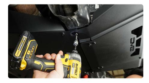
STEP 12 | Use an 18mm socket to secure SPTL4-02's front mounting bolts.
