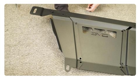
STEP 5 Use a #5 allen tool and 13mm wrench/socket to secure the (10) M8x20m wing bolts.
