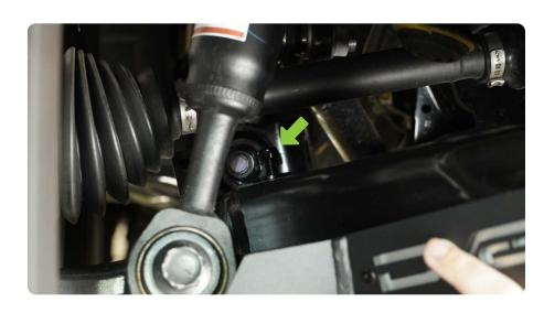
STEP 3 | Install the other (2) M8x110mm carriage bolts and secure them in place using a 13mm wrench and the provided M8 flat washer and nylon lock nut.
