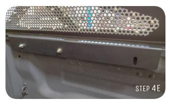
**Note:** Only the 2 front mounting holes on the chase rack are utilized with this mounting method.
