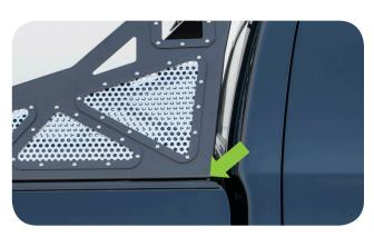
STEP 5E: Now tighten all hardware using an 13mm socket or wrench.
