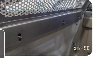
STEP 5D: Using the supplied washers, split washers, and 13mm nuts, tighten finger tight. Repeat on the other side. Then slide the rack forward or backward so it lines up with the front of the bed.
