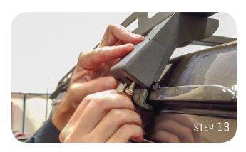
STEP 14: Making sure the rack is centered on the top, tighten up the front and back gutter clamps on each side first. This ensures the 2 other clamps move as needed to fit properly. Then tighten the 2 middle clamps.
