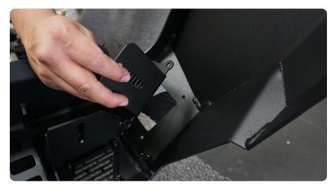
STEP 19 | Install the blind spot monitoring sensors using 3 of the provided "U" Shape spacers on each side.
