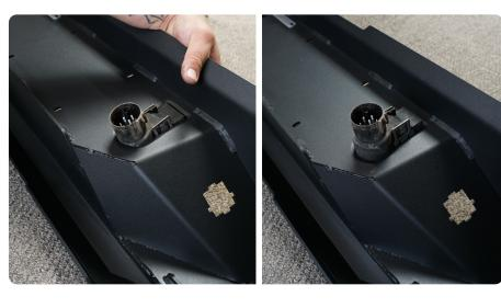
**STEP 22** Insert the factory license plate light housings through the front of the bumper.
