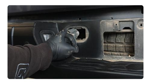
**STEP 4** Unplug the trailer connector socket from the vehicles factory wiring harness by depressing the locking tab on the harness and pulling the plug from the socket.
