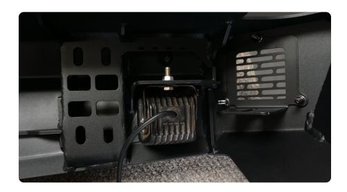
STEP 21 | Insert the trailer connector socket through the front of the bumper.
