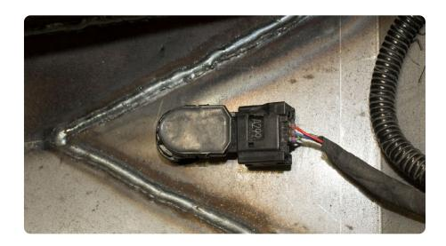
**STEP 24** Connect the license plate light harness to the license plate light housing using the provided zip tie tabs to secure any loose wiring.
