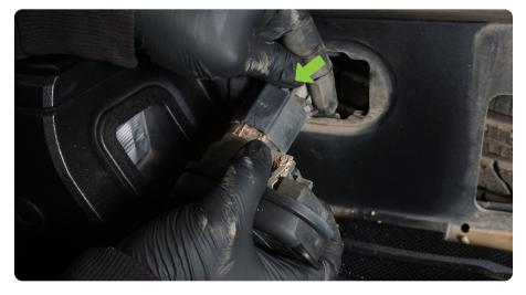
**STEP 5** Continue using trim pry tools to remove the plastic bumper caps from the bumper on both sides.
