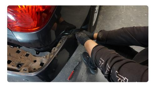
STEP 13 Unplug the blind spot monitoring sensors and using a 10mm socket, remove the BSM sensors.
