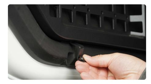
STEP 6 | While holding down the molle pocket, tighten the factory screws using a T15 Torx Bit.
