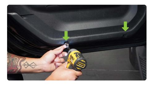
STEP 4 | Slide the DV8 Door Molle Pocket tabs behind the factory door pocket plastic.
