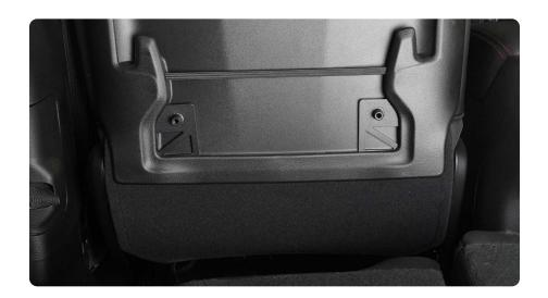
STEP 3 | Attach the Molle Pocket to the mounting tabs using the provided M6 hardware and a #4 Allen tool.
