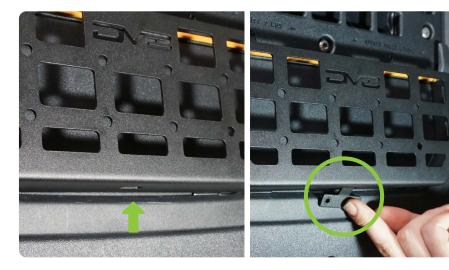
STEP 5 Using a Phillips head screw driver and the provided hardware, secure the mounting tab in place.
