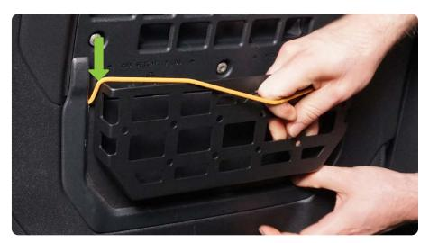
STEP 3 | Ensure the pocket is fully seated at the bottom of the panel and flush with the green line.
