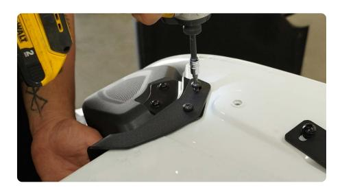
STEP 8 | Hold the dog barrier up under the roll bar, aligning the mounting brackets with the welded nuts on the dog barrier.
