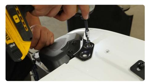
STEP 7 Install the provided rear dog barrier mounting bracket on top of the rear speaker brackets and loosely secure the mounting bracket using the factory hardware.
