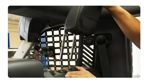
STEP 3 | Slide the provided dog barrier stop brackets on to the head rests as shown with the rubber stop facing toward the rear of the vehicle.
