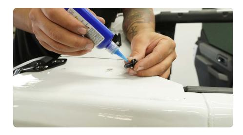
STEP 5 | Loosely install the (2) forward facing upper mounting brackets.
