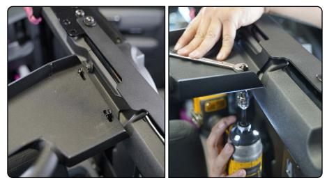
**STEP 15** Use a #5 allen bit to secure the hardware holding the mounting plate to the roll-bar.
