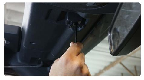
**STEP 10** Use an 8mm wrench to remove the factory roll bar trim bolt.
