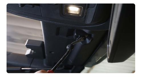
STEP 2 Use a "L" shaped T-20 Torx bit to remove the sun-visor catch for both sun visors.
