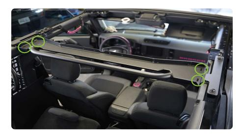
STEP 14 Use a #4 Allen bit and 10mm wrench to secure the M6 hardware holding the cross-brace to the roll bar mounting bracket.
