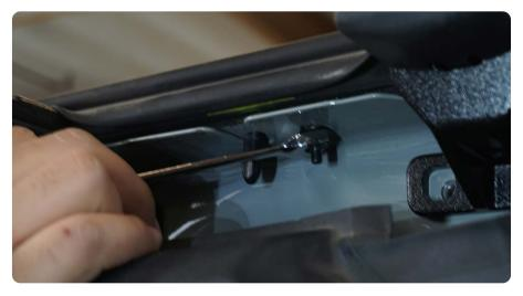
STEP 7 | Install the front mounting bracket as shown and secure using the factory hardware with a T50 Torx bit and a 10mm wrench.
