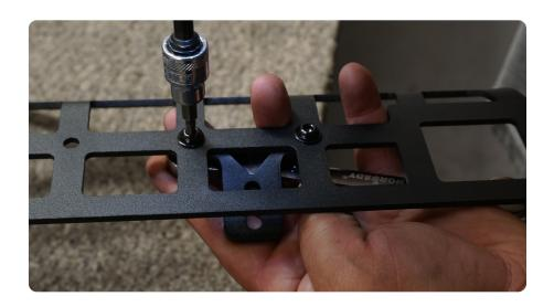
STEP 7 | Once the lower bracket is installed, position the molle panel into the vehicle against the previously installed brackets.
