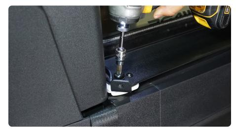
STEP 5 | Lastly, using a #5 allen head and the provided M8 bolt, loosely install the roll bar bracket onto the vehicle.
