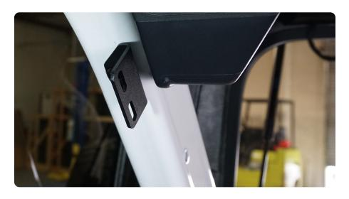
STEP 6 | Moving to the molle panel, install the lower rear bracket onto the panel until secure using the M6 hardware provided a 10mm socket and #4 allen.
