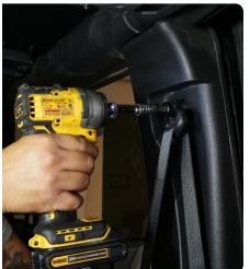
STEP 2 | Using the T50, remove the (3) bolts shown holding the hardtop to the cab.
