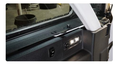
STEP 4 | Loosely Install the forward bracket on the hardtop mount using a T50 torx bit and the factory hardware.
