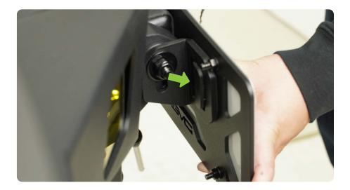
STEP 9 | Insert the locking pin through the license plate tab and into the mounting bracket. Ensure the lock pin is through both pin holes on the mounting bracket to prevent the frame from rattling.
