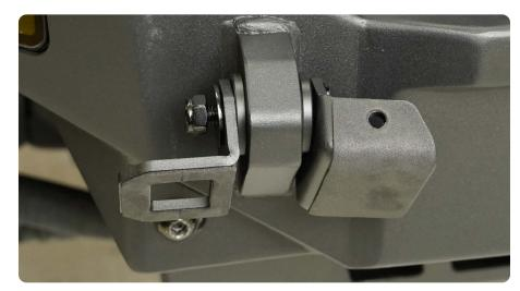
STEP 6 | Use a #6 allen tool and 17mm socket to secure the license plate frame brackets in place.
