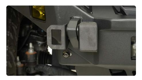
STEP 7 Using a #4 allen tool, 10mm socket/wrench and the provided M6 hardware, secure the license plate to the DV8 license plate frame.
