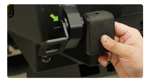
STEP 5 | Use the second provided M10 flat washer and M10 nylon lock nut to loosely secure the license plate frame brackets to the D-ring.
