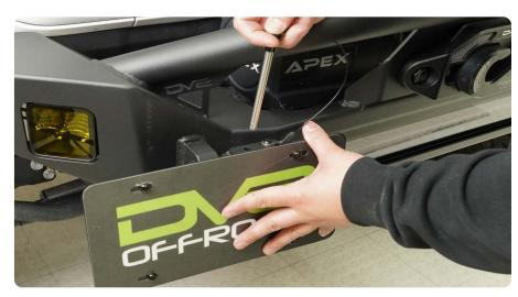
STEP 10 | Once completed, ensure the license plate does not lift up easily or come off. The pin can be ran upside down to hide the pin button.
