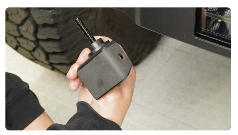
**STEP 3** | Thread the M10 bolt and bushing into the D-ring.
