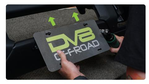
STEP 4 | Raptor owners: Use the provided spacers and M8x40mm hardware to loosely secure the bracket to the bumper. (1 spacer &1 M8 flat washer per M8x 40 Allen head bolt)
