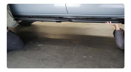
STEP 3 | Once all hardware is loosely installed, center the steps on vehicle and secure the hardware using a 13mm socket.
