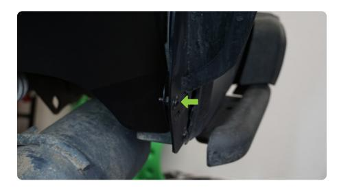
STEP 12 | Use the provided push pin to secure the front of the inner fender to the vehicle.
