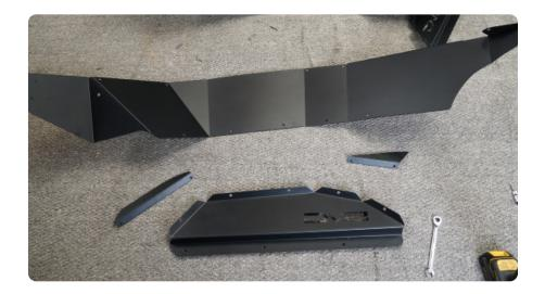
STEP 6 | Lay the large wheel well panel into the center section as shown.
