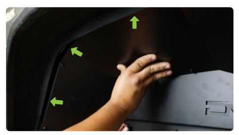
STEP 10 | Use the provided M6x20 hardware to secure the inner fender/center panel to the wheel well.
