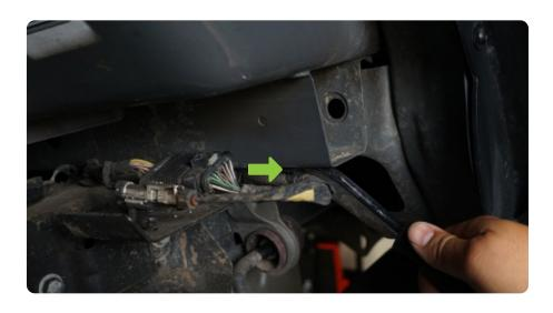
STEP 4 Using a 13mm socket remove the electrical frame brackets from each side.
