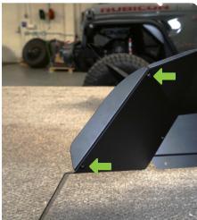
STEP 8 | Install the rear wheel well extension panel behind the large wheel well panel as shown.
