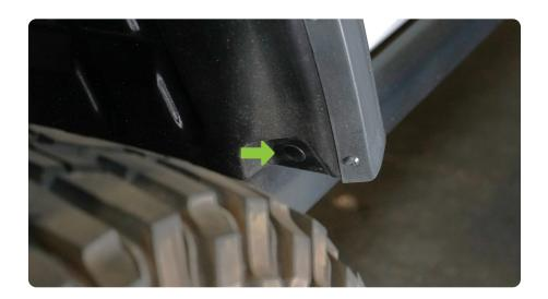
STEP 2 | Use a trim clip tool to pry the (2) plastic rivets securing the factory inner fender to the factory fender flare.
