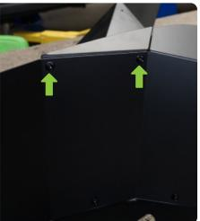
STEP 9 | Place the rear of the inner fender inside the wheel well first, than bring the front section up ensuring all panels are behind the fenders pinch welds.
