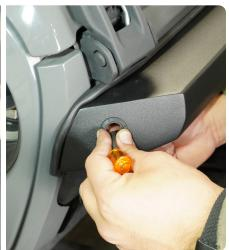
STEP 17 | Press the marker light into the rubber grommet, route the marker light wiring harness behind the inner fender and plug it into the vehicles factory fender/turn single light harness.
