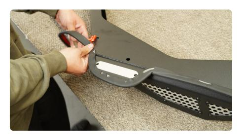
STEP 12 | If planning to bypass vent cover, cut the seal at the fender corner. Continue the seal down the fender aligning the seal cut outs with the mounting holes in the fender. Cut off any excess seal.
