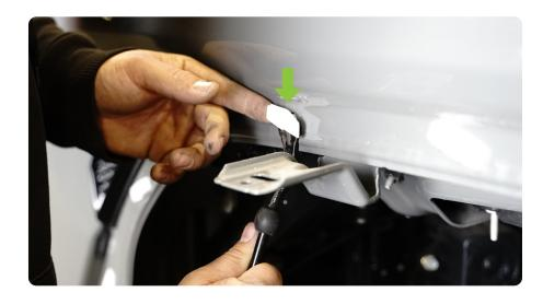
STEP 5 | (Rear uninstall) Use a trim clip tool to remove the clips located along the interior of the inner fender.
