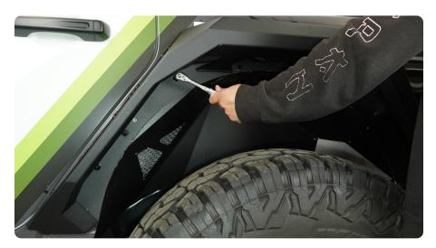
STEP 23 | Double check all hardware is secure on the front and rear fenders.
