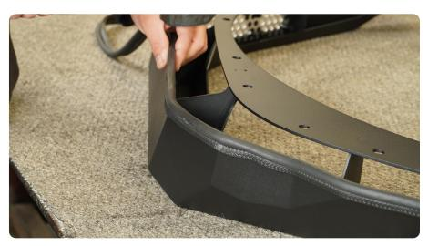
$\begin{array}{c|c} \text{STEP 19} & \text{Cut any excess seal off the} \\ \text{end.} \end{array}$
