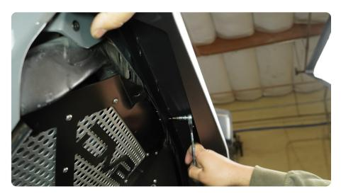
STEP 15 | With all M6x20mm allen bolts started, secure the M6 hardware hand tight using a #4 allen tool.
