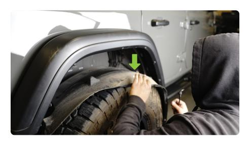
STEP 6 | Remove the fender flare by pulling directly away from the vehicle. Be sure to pull straight away from the vehicle to prevent breaking clips.
