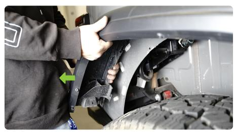
STEP 7 | Use a trim clip tool to remove the clips along the edge of the fender.
