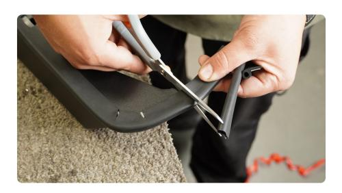
STEP 13 | Remove the factory fender vent cover using a trim clip tool to pry the bottom away from the fender, then slide the cover toward the front of the vehicle to free the cover from the fender.
