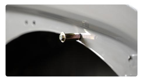
STEP 26 | Use a 12mm wrench to hold the spacer while tightening with a 10mm socket. Tighten slowly until the nutsert is set properly. Do not over tighten.
