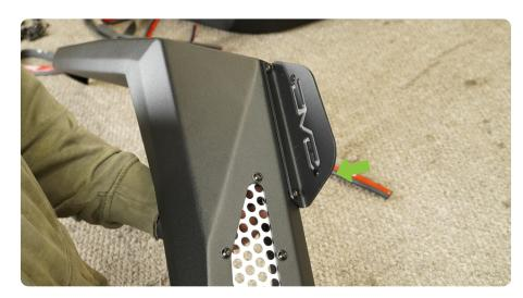
STEP 11 | Place the peel-N-stick rubber seal onto the back of the fender, aligning the cutout in the seal with the fender mounting bolt holes.
