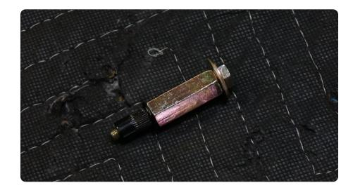
STEP 25 | Slide the nutsert tool with the nutsert into the mounting hole. Ensure the flange of the nutsert is flat against the vehicle prior to tightening.
