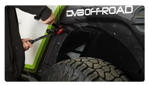
STEP 21 | Lift the rear fender up to the vehicle and loosely secure the fender to the vehicle using the provided M6x20mm allen head bolts.
