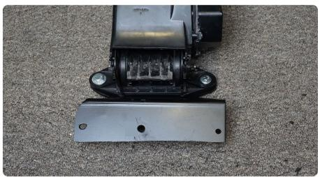
STEP 34 | Install the air dam bracket onto the horizontal cross brace using the provided M6 hardware and a 4mm allen bit. Connect the air dam motor wiring plug.
