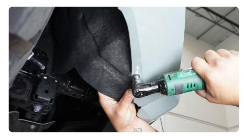
STEP 43 | Attache the Bumper support brackets using a 5mm Allen bit, a 13mm wrench and the provided M8 hardware.
