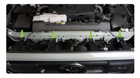
STEP 45 | Install all push pins and reconnect all wiring harness's previously removed or disconnected.
