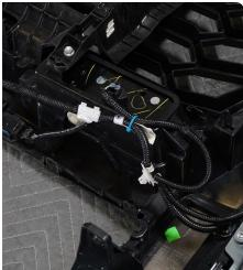
STEP 18 | With the bumper face removed and wiring harness's secured out of the way, use a marker to draw a cut line.
