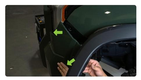
STEP 3 | Reach behind and underneath the bumper to remove the black plastic trim by pressing out the clips from the inside.
