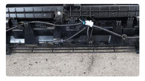
STEP 20 Using a 5mm Allen bit, 13mm wrench and provided M8 hardware attach the bumper support brackets to each side of the DV8 center mount.
