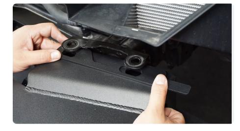
Using a 21mm socket, 22mm wrench and provided M14 hardware secure the spacer plates to the center mount.
