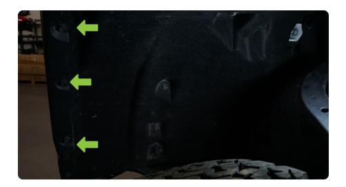
STEP 2 | Using firm pressure, pull the fender flare away from the truck to the side to release the clips.
