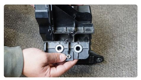
STEP 27 | Trim the small remaining mounting tab off the motor as shown.
