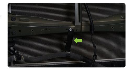
STEP 13 | Use a 12mm socket to remove the bolts securing the skid plate if you have one, and set it off to the side.
