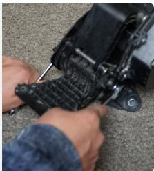
STEP 23 | Remove the black caps, the white plastic spacers and the spring from the inside, and set the arm off to the side.
