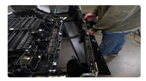
STEP 16 Using a Pry Tool, unclip the 5 wiring harness hold downs.
