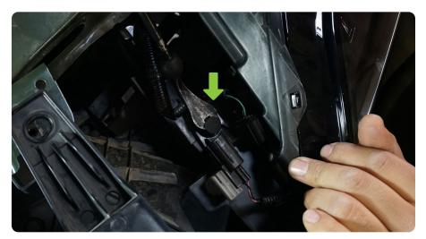
STEP 7 Disconnect the wiring plugs located behind the grille on the passenger side of the vehicle underneath the grille's upper mounts.
