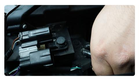
STEP 5 | Disconnect the wiring plug located between the bumper and radiator in the center section of the vehicle.
