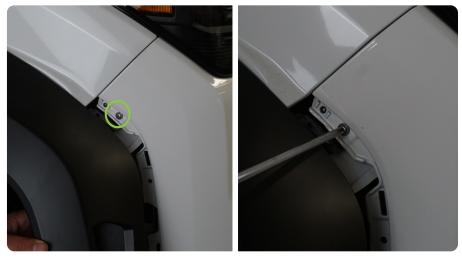
**STEP 8** Use a 10mm socket to remove the bolts securing the lower bumper valance.
