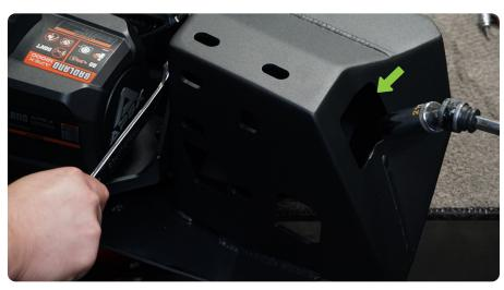
**STEP 11** | With assistance lift the bumper into place.
