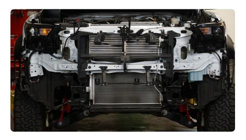
STEP 2 | With the factory bumper removed it is now time to build out the DV8 Centric Front Bumper.
