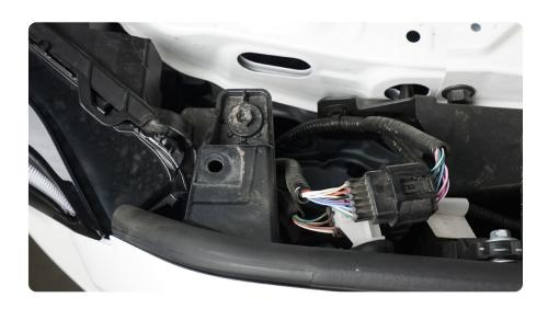
STEP 22 | Reinstall the radiator support cover and intake fresh air duct using the factory push pins.
