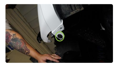
STEP 7 Pull the front of the fender flare down to expose the Phillips head screw securing the side of the front bumper to the vehicle. Use a Phillips head screw driver to remove the screw from each side.
