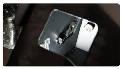
STEP 20 | Reinstall the bumper/ grille, snap in all front bumper/grille clips and reinstall the Phillips head screw on each side.
