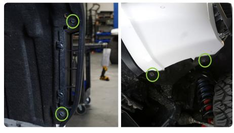
**STEP 5** Use a trim pry tool to remove the (2) push pins on each side securing the factory flare to the bumper (If equipped).
