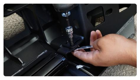
STEP 5 | Install the pod lights using the hardware provided with the light.
