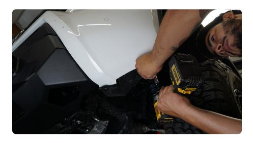
STEP 24 Clip in the factory fender flares (if equipped). Reinstall the (2) factory 10mm bolts that secure the inner fender to the fender flare on each side.
