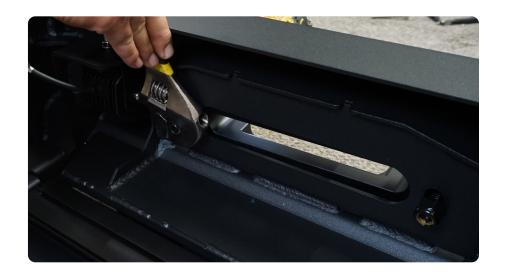
**STEP 7** | If running a winch, mount the winch to the provided winch plate at this time using the hardware provided with the winch.
