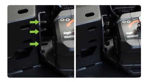
STEP 10 Use a 22mm wrench and 21mm socket to secure the (6) winch plate mounting bolts.
