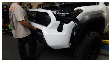
STEP 1 Use a 17mm socket to remove the (8) bolts securing the crash bar.
