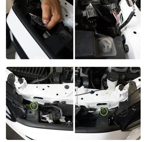
**STEP 3** Use a 10mm socket to remove the (3) bolts securing the top of the grille to the vehicle.
