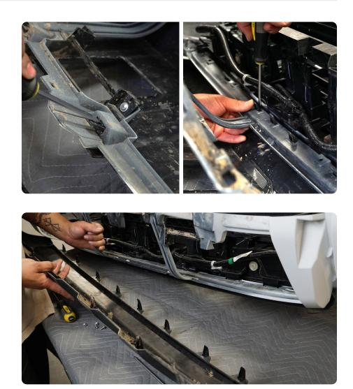
**STEP 15** Using your preferred cutting tool, cut the bumpers center section following along the inner edge as shown with our yellow guide line.
