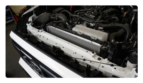
STEP 2 | Disconnect the 2 electrical plugs connected to the grille.
