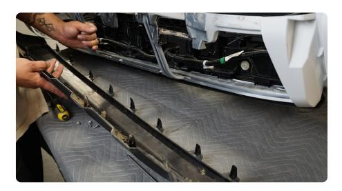
STEP 25 Using your preferred cutting tool, cut the bumpers center section following along the inner edge as shown with our yellow guide line.
