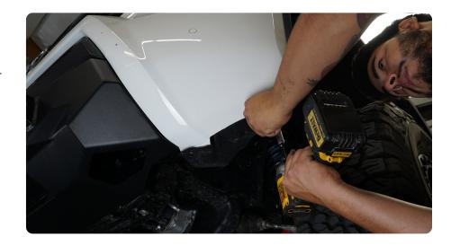
STEP 34 | Clip in the factory fender flares (if equipped). Reinstall the (2) factory 10mm bolts that secure the inner fender to the fender flare on each side.
