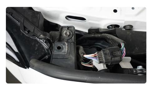
STEP 32 | Reinstall the radiator support cover and intake fresh air duct using the factory push pins.
