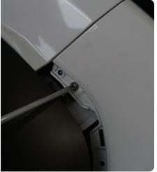
STEP 8 Use a 10mm socket to remove the (2) bolts securing the lower bumper valance.
