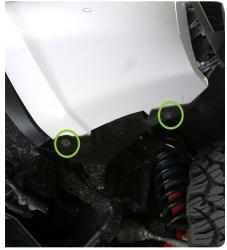
STEP 5 Use a trim pry tool to remove the (2) push pins on each side securing the factory flare to the bumper (If equipped).
