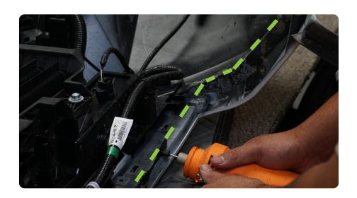
$\begin{array}{c|c} \text{STEP 26} & \text{After initial cut, install the} \\ \text{front bumper/grille on the vehicle loosely.} \end{array}$
