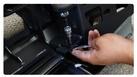
$\begin{array}{c|c} \text{STEP 15} & \text{Install the pod lights using} \\ \text{the hardware provided with the light.} \end{array}$
