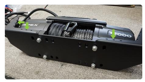
$\begin{array}{c|c} \text{STEP 18} & \text{Route a portion the winch} \\ \text{rope through the fair-lead.} \end{array}$
