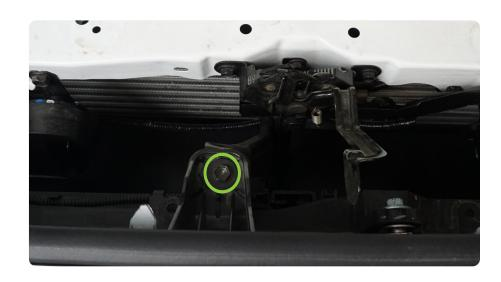
STEP 4 Use a 10mm socket to remove the (4) bolts on each side securing the inner fender to the front bumper.
