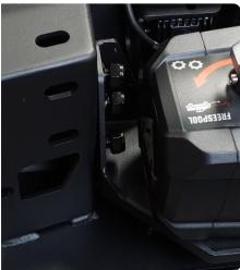
STEP 20 | Use a 22mm wrench and 21mm socket to secure the (6) winch plate mounting bolts.
