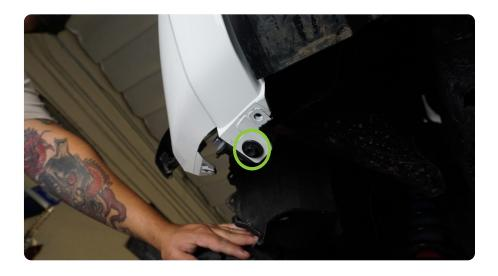
STEP 7 | Pull the front of the fender flare down to expose the Phillips head screw securing the side of the front bumper to the vehicle. Use a Phillips head screw driver to remove the screw from each side.
