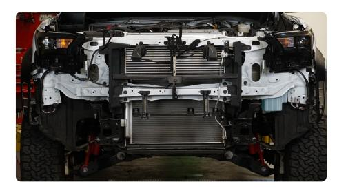
STEP 12 | With the factory bumper removed it is now time to build out the DV8 Centric Front Bumper.
