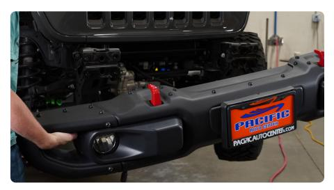
STEP 5 | At this point, frame rails should be visible and the vehicle should as shown.
