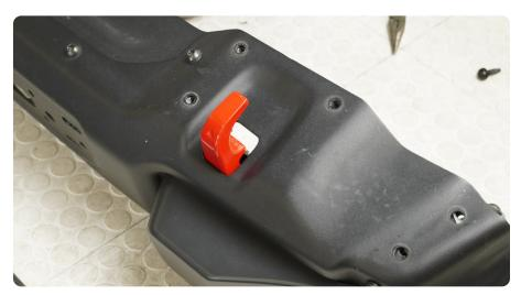
STEP 7 Use a T45 torx tool to remove the (5) torx head bolts at the bottom of the bumper from each side.
