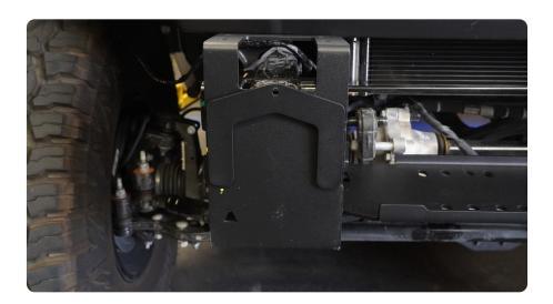
STEP 16 | If you are running a winch with a larger housing such as a Badlands or Warn winch (will vary), use the provided spacer plates between the factory frame rail brackets and the DV8 bumper mounting brackets as shown.
