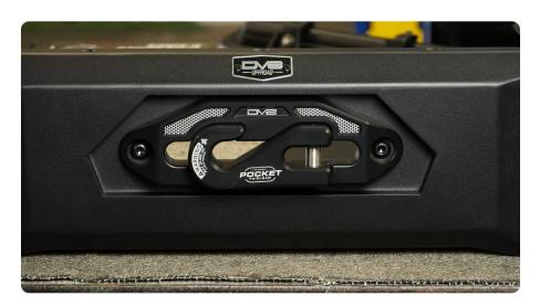
STEP 23 | If you are not running a winch, install the winch cover plate at this time.
