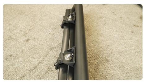
STEP 32 | If you are mounting a DV8 Elite LED light bar you will need use the DV8 elite series light bar mounts (part# BESLDBKTSM) as shown.
