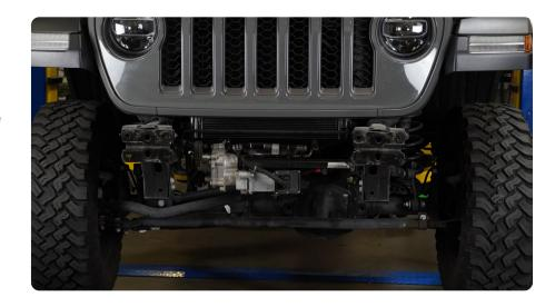
STEP 12 | If you are planning to run a winch, install the winch mounting plate at this time as shown, letting the winch plate rest on the inside frame rail brackets.
