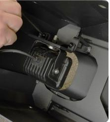
STEP 22 | If you are running a winch, install the winch fairlead at this time using the hardware provided with the fairlead.
