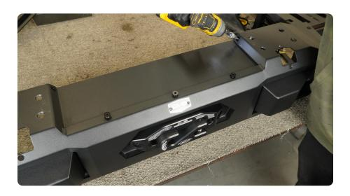
STEP 24 | To install the bumper with the factory recovery hooks mounted, place the bumper over the recovery hooks at an angle as shown. Press the bumper down and over the factory recovery hooks until the bumper wraps fully around the bumper mounting brackets.
