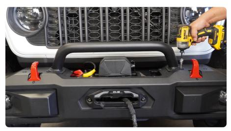
STEP 28 | Secure the bottom of the bumper to the bumper brackets using the provided M10x25 allen button head bolts and a #6 allen tool.
