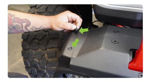
STEP 30 | Use the provide M8x25 counter sunk allen head bolts and M8 nylon lock nuts to loosely secure the bumper wings to the bumper.
