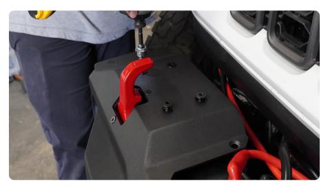
STEP 26 | If you are not running the factory recovery hooks, place the bumper straight onto the bumper mounting brackets and secure the bumper.
