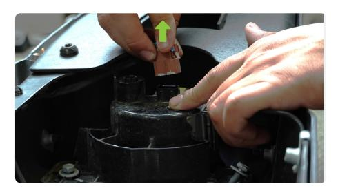
STEP 7 | Remove the fog lights from the factory bumper and set them to the side for installation on the DV8 bumper.
