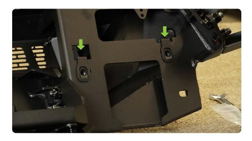
STEP 20 | If you are planning to run LED Pod lights, install them at this time, using the hardware that is provide with the light.
