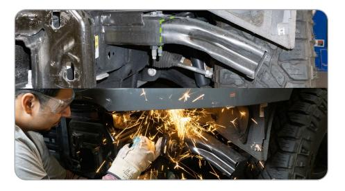
**STEP 8** | If your bumper is equipped from the factory with front parking sensors, begin by removing the automatic air dampening system on the factory bumper using a 13mm socket on the three bolts located on each side.
