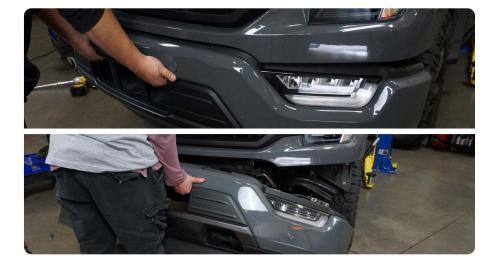
STEP 4 Disconnect the lower shutter motor and the electrical plug on top of the lower shutter assembly. Use a trim clip tool to remove any harness clips.
