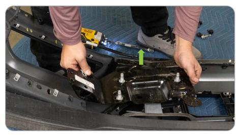
STEP 11 | If you have an adaptive cruise control (ACC) module, unplug this off the driver side bracket and set off to the side since this will not be a part of the bumper install.
