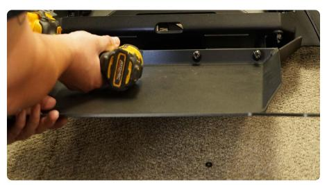
STEP 26 | Moving to the shutter motor removed earlier, start by assembling the installed shutter stops.
