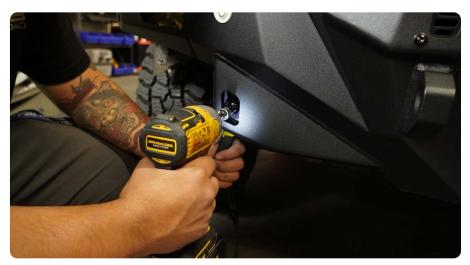
STEP 41 | Using the 13mm socket, reinstall the rear skid plate over the DV8 skid plate and secure using the factory hardware.
