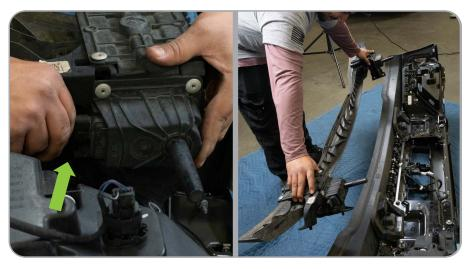
**STEP 9** Using a T30 torx bit, remove the four bolts holding fog light housing on each side of the factory bumper. Unplug the fog lights and set off to the side.
