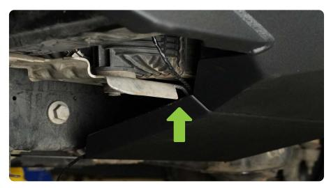
**STEP 40** Adjust bumper side to side/ up and down and using a 18mm socket, secure the 4 bolts (2 per side) on the frame horns.
