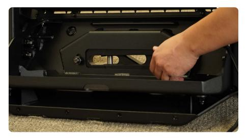
**STEP 24** | Install your winch at this time. Secure the winch to the winch plate using the hard that is provided with your chosen winch.
