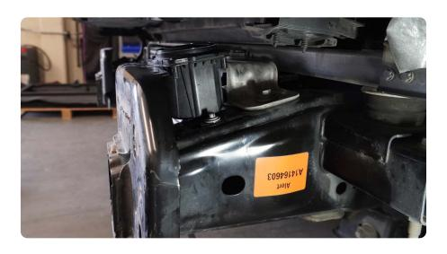
**STEP 38** With assistance, life the bumper into place and loosely secure the bumper onto the truck using the M12 hardware supplied.
