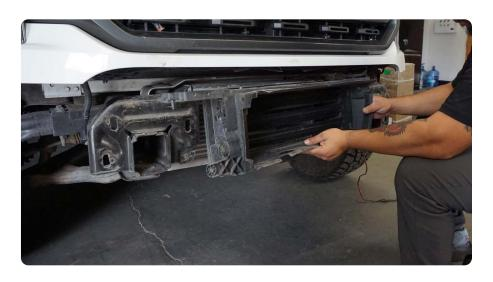
STEP 6 Use a T20 Torx tool to remove the lower shutter motor and set it off to the side to be reinstalled onto the DV8 Spec Series front bumper.
