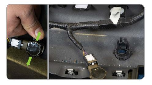
**STEP 13** Using the push pin tool, remove the harness from all points on the factory bumper.
