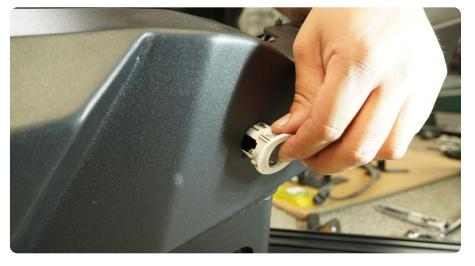
**STEP 33** Start feeding the harness into the bumper. Each sensor plug should land near the bezel placed before.
