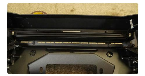
**STEP 23** Install your chosen fair lead at this time using the hardware provided with the fair lead.
