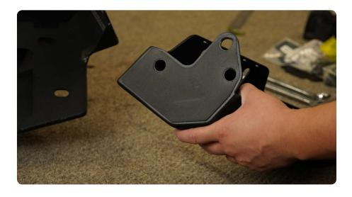
STEP 16 | Attach each bumper wing using (3) of the provided M12 hardware. Use a 21mm and 22mm wrench to loosely secure the wings in place.
