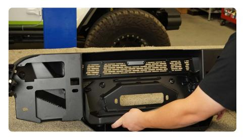
STEP 18 | Use a 21mm socket and 22mm wrench to secure the (4) hex bolts. Use a #6 allen tool and 17mm socket to secure the rear (2) Allen head bolts.
