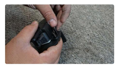
STEP 29 | Lastly, place the gear stop bracket over the gear bolt and secure using a #4 and 10mm socket/wrench.
