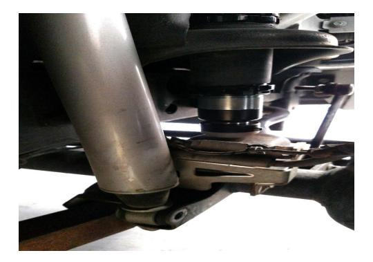
Take notice of the relationship between the shock and the bump stop. It is ideal for the shock to have between  $\frac{1}{2}$  to  $\frac{3}{4}$  of an inch of shaft exposed with the bump stop being completely bottomed out.
