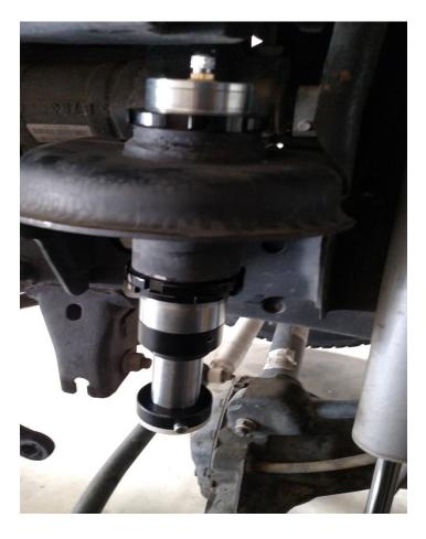
Slide the new hydraulic bump in the factory bump stop tube. With stepped ring pointing up in the lower tube. Adjust bottom stop to its lowest setting. Leave lock rings loose at this time.
