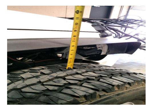
Make sure you have proper tire clearance with the vehicle completely bottomed out.
