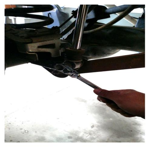
With the frame and axle housing supported carefully remove the lower front shock mounting Hardware. Be sure to support the axle at this time in order to keep the axle from dropping Out suddenly.
