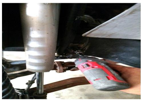
With the housing still supported remove brake line bracket hardware.
