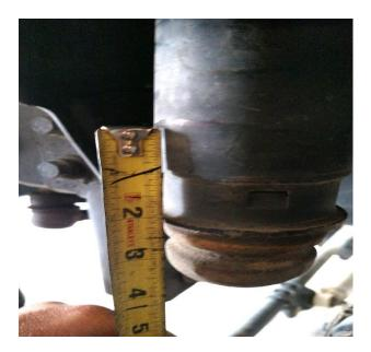
With the coil spring removed carefully measure the factory bump stop mount. Using a marker or scribe mark the measurement at 2 inches from the lower bump stop rib Using a sawsall or similar cutting tool cut on your mark. Be extra cautious that your cut be even and flat from front to back. Once the piece is cut remove it and check for burrs inside of the bump mount. Remove any burrs if present.
