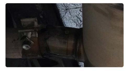
STEP 16 | Finish securing the muffler by re-installing it onto the hangers.
