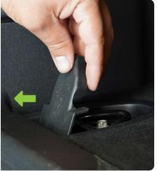
STEP 4 Use a 10mm socket to remove the hardware securing the factory tie-downs to the vehicle.
