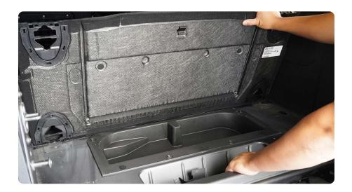
STEP 6 Use a 10mm socket to remove the hardware securing the factory storage box to the vehicle.
