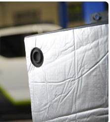
STEP 3 | Use a trim clip tool to remove the plastic covers from the tiedown hooks.
