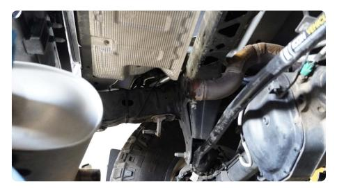
STEP 10 Use a 10mm socket and a trim clip tool to remove the factory hardware and plastic clip retainers securing the factory heat shield in place.
