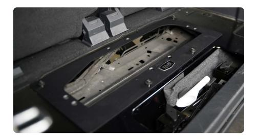
STEP 12 | Place the DV8 storage box under the vehicle and lift it to the mounting plate by reaching down through the empty space in the cab.
