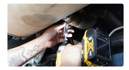
STEP 18 | Install factory tie-downs using a 10mm socket and the factory hardware.
