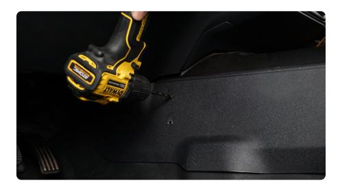
STEP 3 Align the driver side mount with the mounting holes and press the M6x15 hardware into the drilled out holes, to loosely hold the mount in place. Pull back on the center console trim from the bottom to fit the M6 nuts into place.
