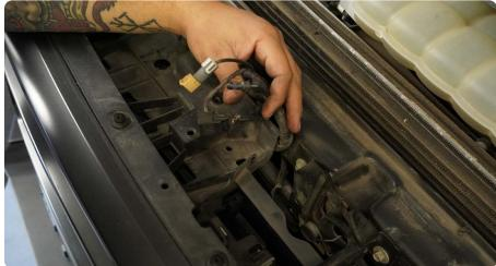
**STEP 16** With a firm grip pull on the sides of the grille to pop the retaining clips. Remove the grille assembly and place on a covered work bench or on blanket face down to protect the paint finish.
