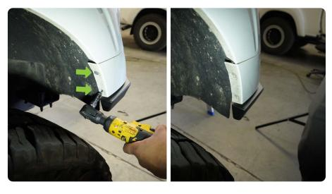
**STEP 13** | With a firm grip, remove the lower fascia from the vehicle.
