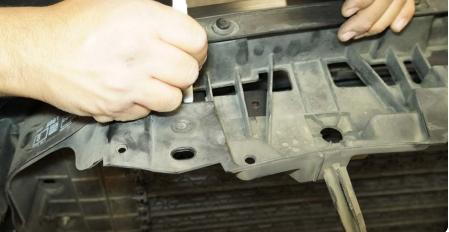
STEP 18 | Remove the drilling template and use a 1/4" drill bit to drill out the (2) mounting holes
