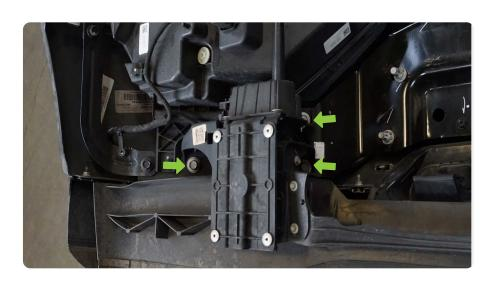
**STEP 4** Use a T30 torx tool to remove the (4 per side) fog light assembly bolts.
