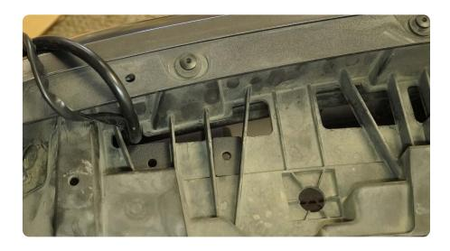
STEP 25 | Mount the upper portion of the bracket onto the grille as shown. Make sure the hex head M6 hardware is facing down. Be sure to mount the bracket with (2) of the provided spacers between the grille and shutter.
