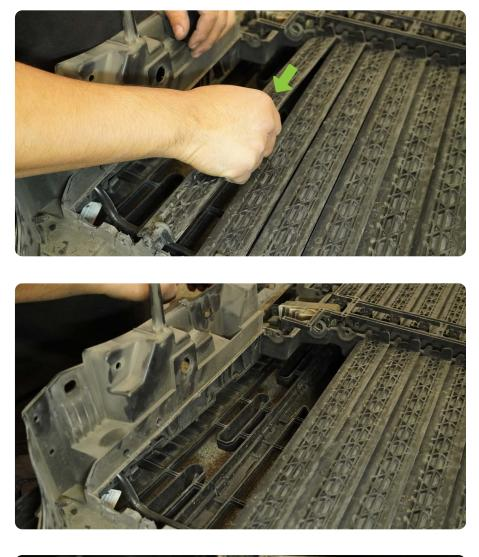
**STEP 21** Use your preferred cutting tool to make a small notch at the bottom and in the middle of the grille assembly as shown to route the
