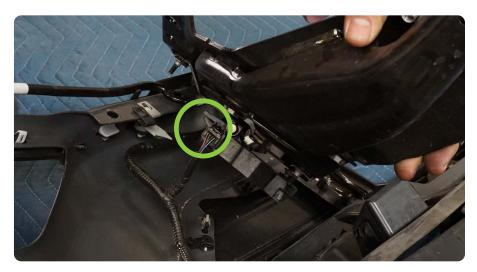
**STEP 6** | Remove the ACC module by depressing the retaining clip and sliding the module down.
