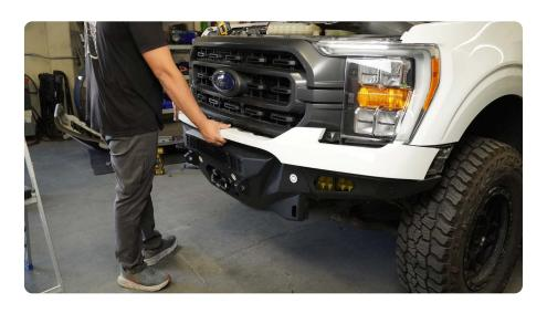
STEP 14 | Use a 8mm socket to remove the (2) lower bolts securing the grille.
