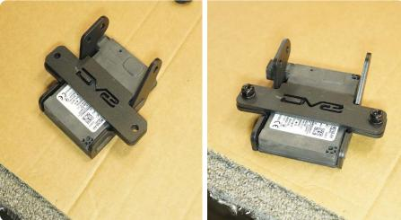
STEP 23 Use a #4 Allen tool and a 10mm socket/wrench to secure the M6 hardware.
