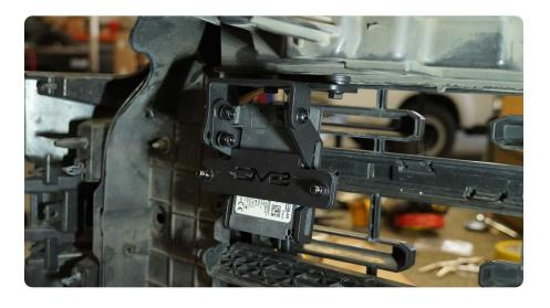
STEP 27 | Adjust the tilt on your ACC module so that the module is parallel to the front face of the grille, and perpendicular to the ground. Secure the ACC module hardware in place using a #4 Allen tool and 10mm socket/wrench.
