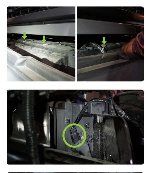
STEP 3 Remove the factory front bumper and set face down on a work bench, disconnect the spoiler system and use a 13mm socket to remove the (3) bolts per side that secures the factory spoiler system.
