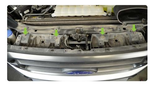
STEP 12 | Use a 6mm socket to remove the (2) bolts securing the lower fascia to the fender-well.
