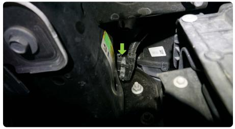
**STEP 1** Disconnect the main bumper harness connector located along the top side of the passenger side frame rail.
